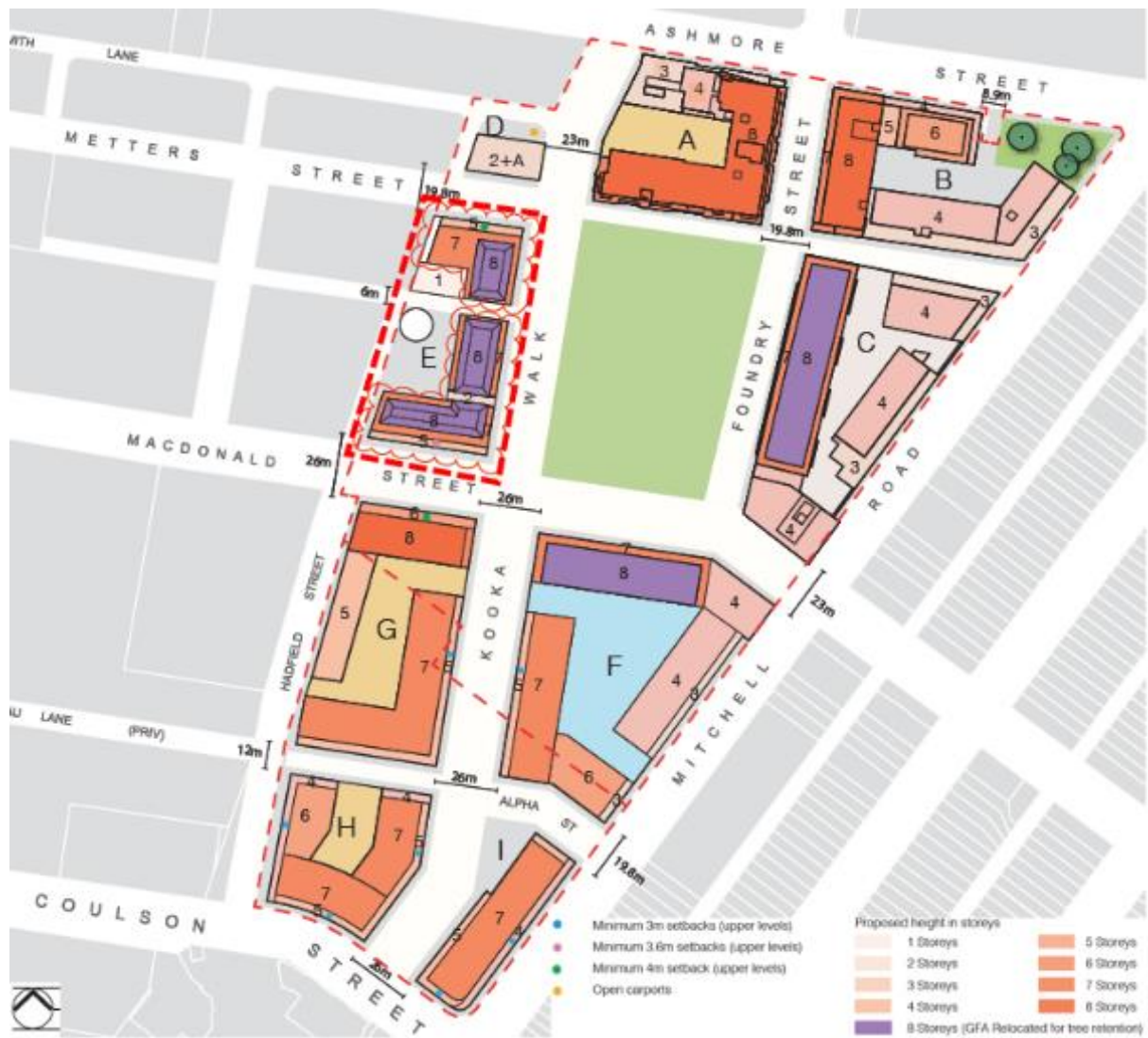
Figure 17: Proposed building envelopes plan (Block E - outlined by red dashed lines and clouded)
