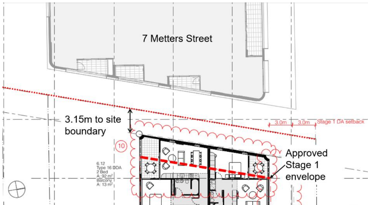
Figure 30: Proposed floor plan - Level 6 of Block E (D/2023/842), depicting separation to side boundary with 7 Metters Street
